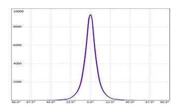
LED Lamp1Luminous Flux1456 lmColour temperature3000 KCRI80MacAdam Ellipse3 StepNominal Power10WBeam Angle12°
