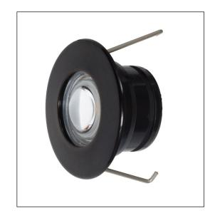
**LED Lamp** Luminous Flux 100 lm 3000 K **Colour temperature** CRI 80 MacAdam Ellipse 3 Step **Nominal Power** 1.6W **Beam Angle** 90°
