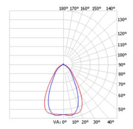
LED Lamp1Luminous Flux100 lmColour temperature4000 KCRI80MacAdam Ellipse3 StepNominal Power1WBeam Angle70°
