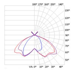
**LED Lamp** Luminous Flux 9245 lm 3000 K Colour temperature CRI 80 3 Step MacAdam Ellipse Nominal Power 80W **Beam Angle** Asymmetrical
