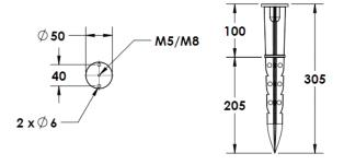
Cast Stirrup Powder coated die cast aluminium
