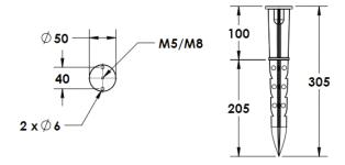
Cast Stirrup Powder coated die cast aluminium
