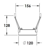
IP65 Gear Base Powder coated die cast aluminium
