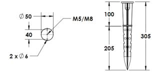
Cast Stirrup Powder coated die cast aluminium
