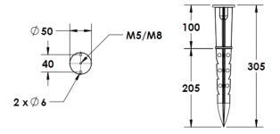
Cast Stirrup Powder coated die cast aluminium
