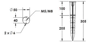
Cast Stirrup Powder coated die cast aluminium
