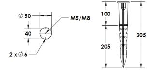
Cast Stirrup Powder coated die cast aluminium
