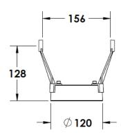
IP65 Gear Base Powder coated die cast aluminium
