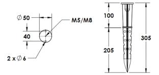
Cast Stirrup Powder coated die cast aluminium
