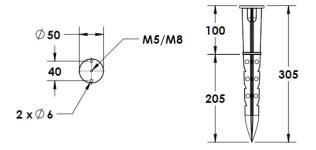
Cast Stirrup Powder coated die cast aluminium
