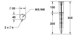
Cast Stirrup Powder coated die cast aluminium
