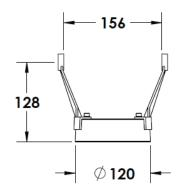
IP65 Gear Base Powder coated die cast aluminium
