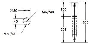
Cast Stirrup Powder coated die cast aluminium
