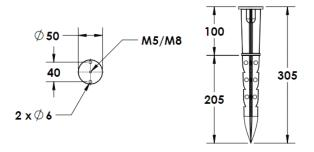
Cast Stirrup Powder coated die cast aluminium
