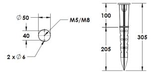
Cast Stirrup Powder coated die cast aluminium
